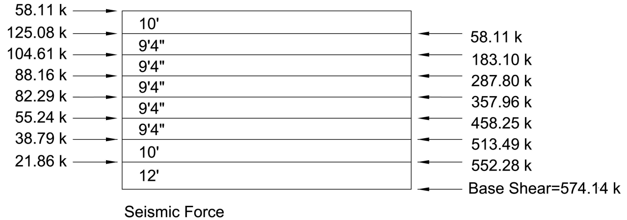
Figure 15: Diagram of Seismic Design Story Shear Forces (Existing Structure)
